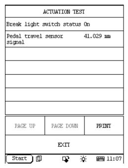
If Pedal travel sensor signal value is below 0.8mm, you should adjust the switch, then perform above steps again until the value is correct.
